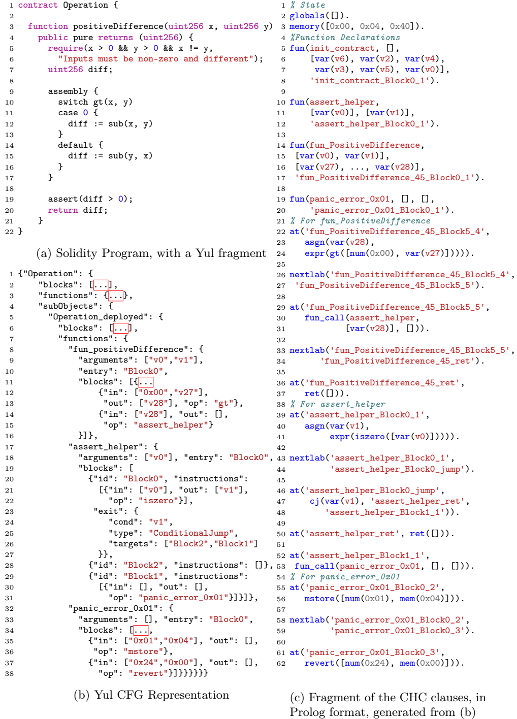
Fig. 2: Diagram showing the different representations of the source program in our framework. For (b) and (c), only a fragment of the translation is shown.
